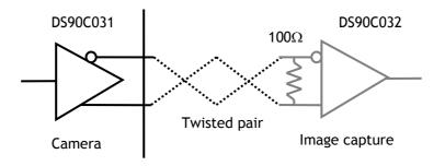
Fig. 5. Output driver circuit for Video, STROBE and LEN signals
